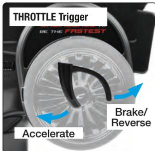
1. Gently pull the throttle trigger to move your model forward.
